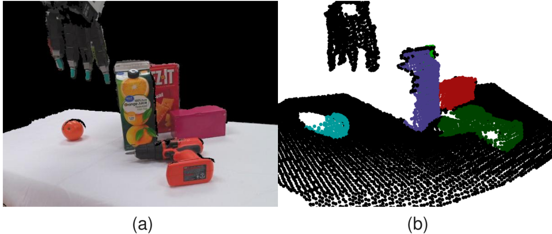
Figure 1: (a) An example RGB image of a tabletop scene. (b) A segmented point cloud of the same scene.
